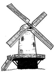
Wilton Windmill is a Tower Mill built as a round brick tower. and again the cap and sails can turn round. These mills could be taller and could hold even machinery. more Wilton Windmill has a fantail at the back which turns the mill to face the wind automatically.
