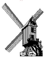
The earliest mills in Britain were called **Post**Mills. A tall post stuck up from the ground and the whole mill body was supported on this post. The body had to be turned round on this post to face the wind. There are still a few working post mills left in this country.
