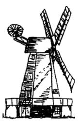
The next type of mill to be built was the Smock Mill. This had a fixed wooden body. The cap and sails on the top were the only bit that turned to the wind. face Smock mills were often bigger than post mills and could hold more bits machinery.
